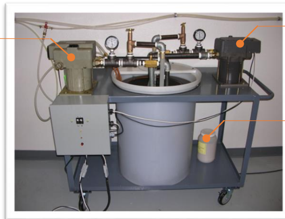
Grit test stand to validate ceramic bearings
