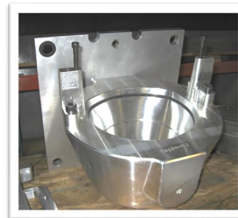
Tail cone vacuum machining fixture
