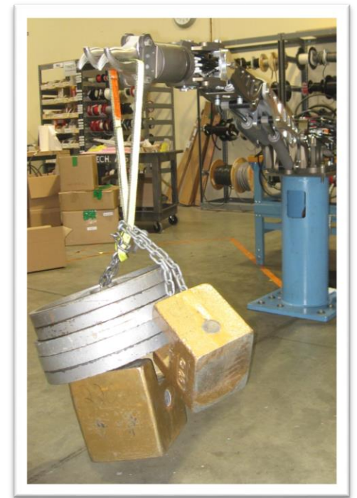
Load tested to 550 pounds at full extension
